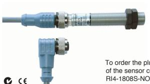
Most of the Rhomberg proximity sensors are now available in "plug" versions. This means that the sensor is supplied with a male plug instead of a moulded lead. The lead is supplied as a separate part. If the sensor requires replacement, simply unplug the old one from the lead and plug the new sensor in.
